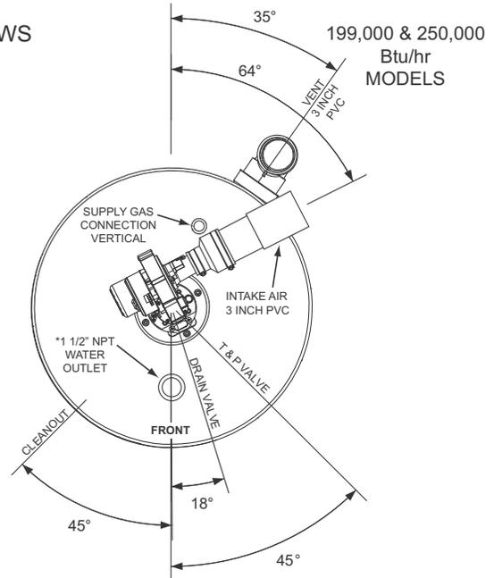
\* Center line of water outlet on top of the water heaters is approximately 7 inches from the front edge of the water heater.
