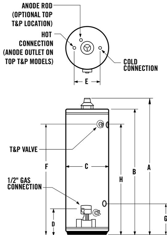
Maximum Hydrostatic Working Pressure: 150 PSI
