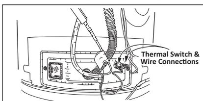
Figure 51 - Thermal Switch and Wire Connections
