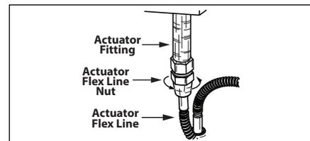
Figure 58 - Actuator Flex Line Connection
