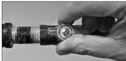
Figure 31 - Gas valve in "on" position
