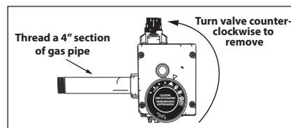
Figure 53 - Removing Existing Gas Valve
