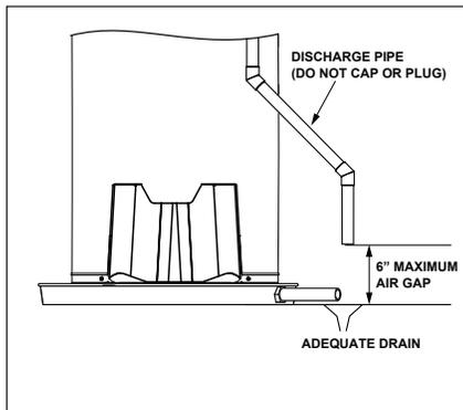
Figure 25 - Temperature and Pressure Relief Valve Pipe
