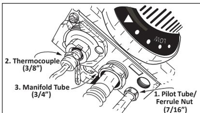
Figure 50 - Component Removal
