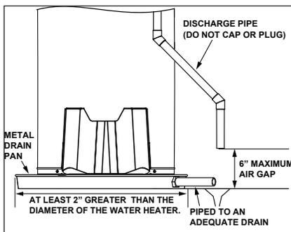
Figure 23 - Metal drain pan piped to drain.
