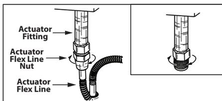
Figure 49 - Actuator Flex Line Removal
