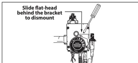
Figure 48 - Igniter with bracket dismount
