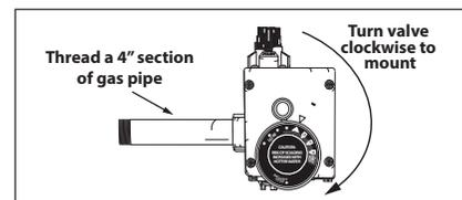
Figure 54 - Installing New Gas Valve
