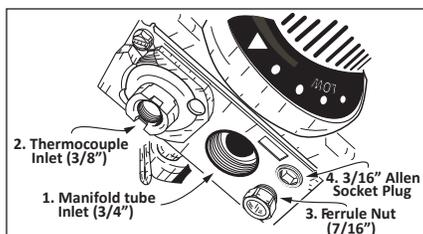
Figure 55 - New Gas Valve Ferrule Nut Removal
