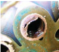
Picture shows a clean HX with treatment.
