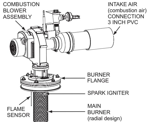
Figure 2. SUF Blower/Burner Components
