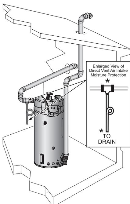
Figure 46. Direct Vent Vertical Vent Horizontal Intake
