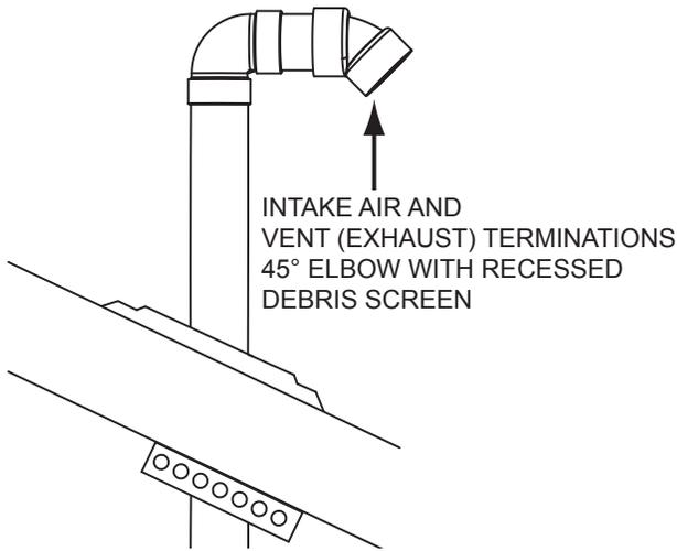
**Figure 21. Standard Factory Supplied Terminations**
