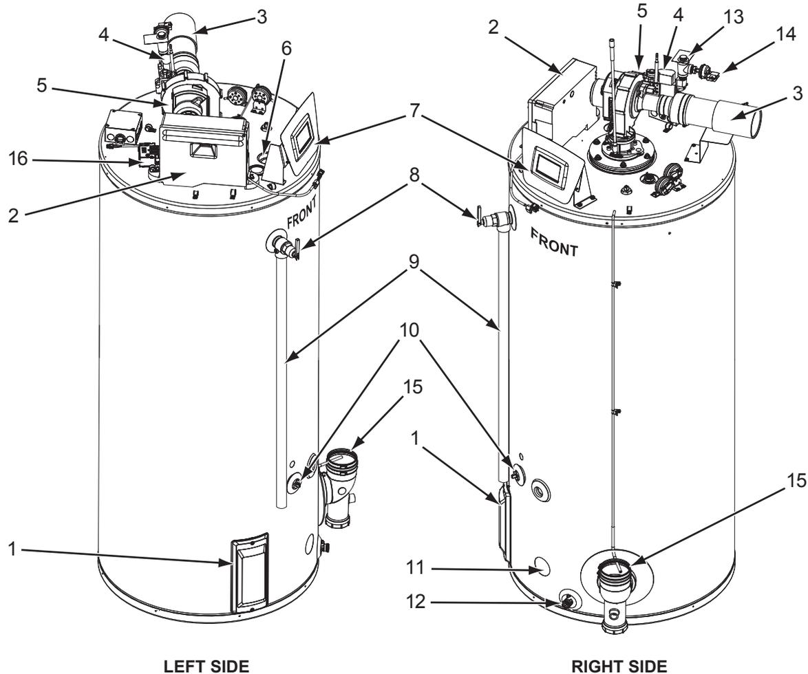
Figure 4. Left-Side and Right-Side Components
