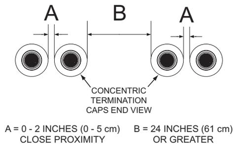
**Figure 34. Four Concentric Terminations**
