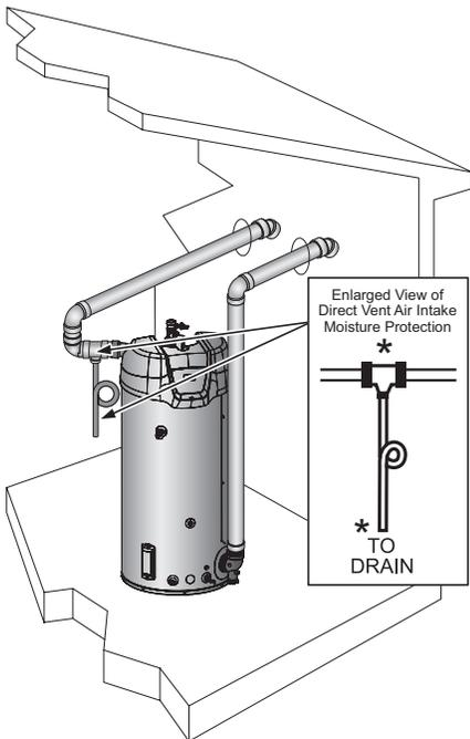
Figure 45. Direct Vent Horizontal
