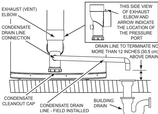
Figure 8. Exhaust/Condensate Elbow
