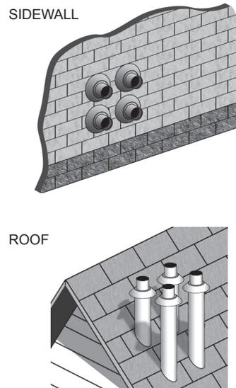
Figure 37. Four Concentric Terminations (Side-Wall and Roof)
