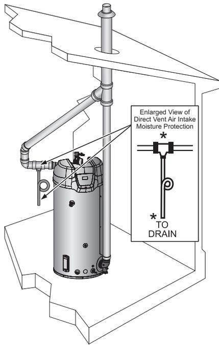
Figure 48. Direct Vent Vertical Concentric
