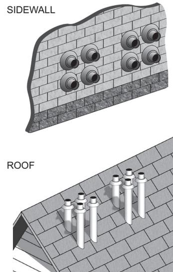
Figure 38. Eight Concentric Terminations (Side-Wall and Roof)
