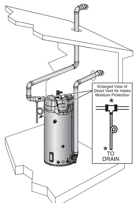
Figure 47. Direct Vent Horizontal Vent Vertical Intake
