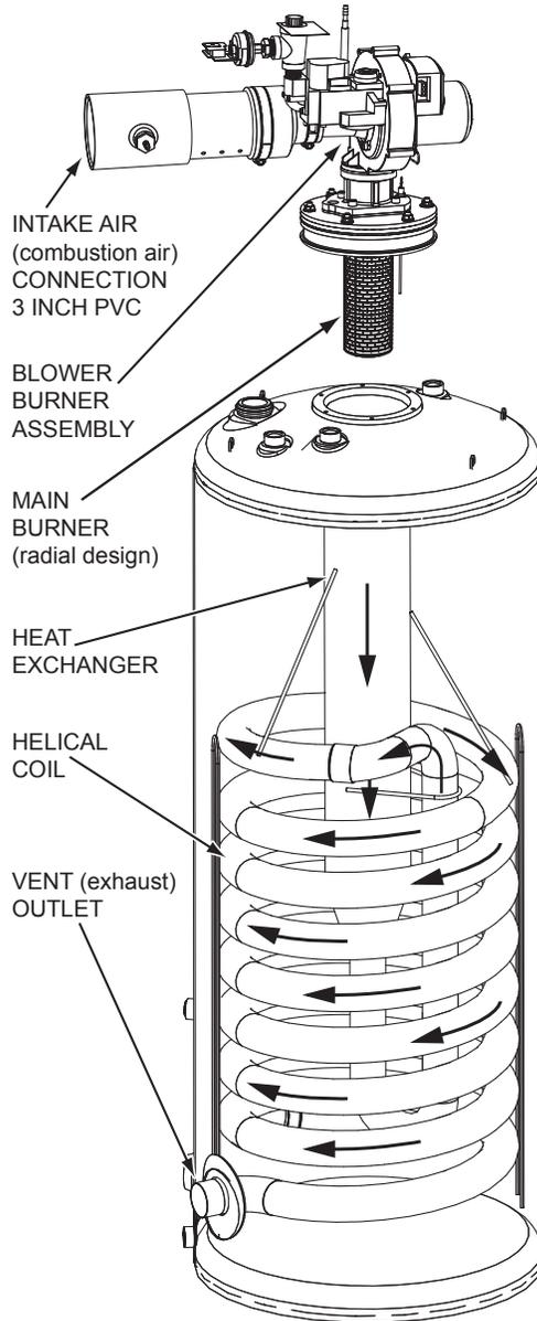
Figure 1. SUF Water Heater Components
