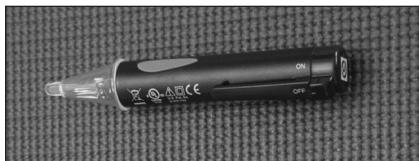
Figure 2 - Use a non-contact circuit tester to ensure that the power is off before you work on a circuit.
